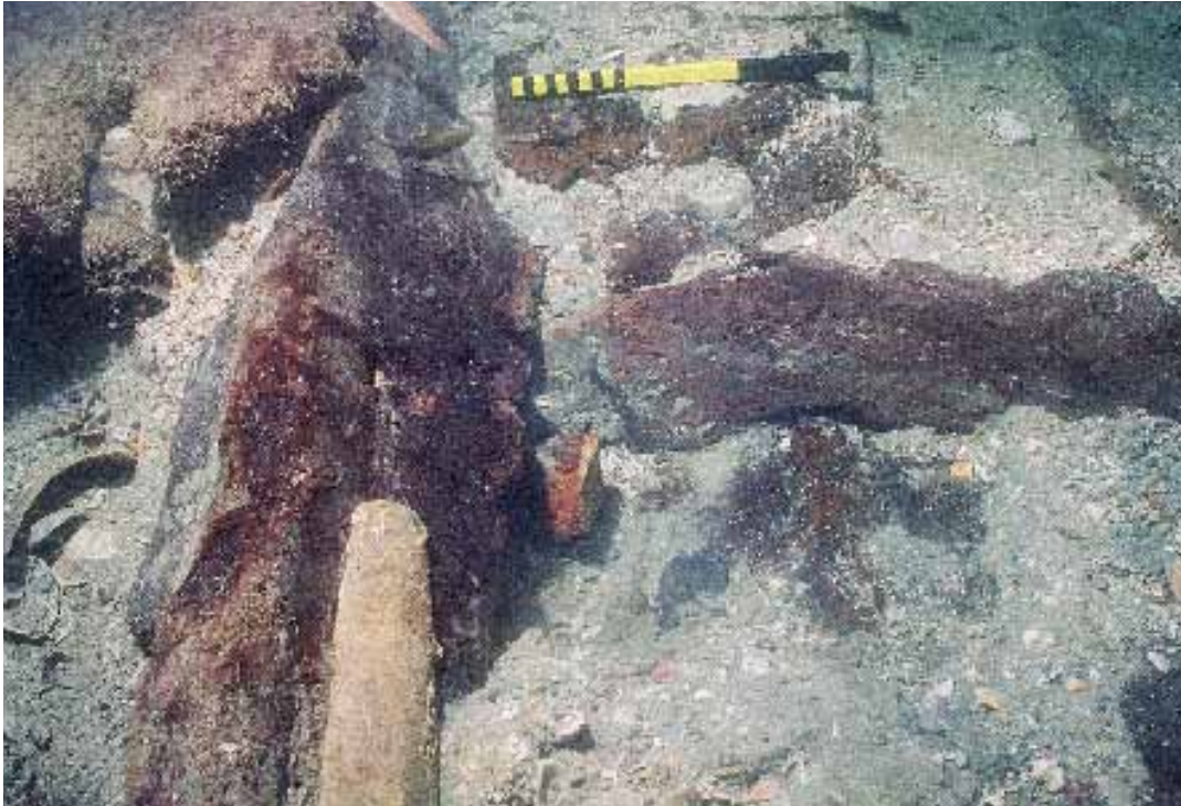
Fig. 79 A curved frame underlying the keelson, which is canted 45 degrees to port.
